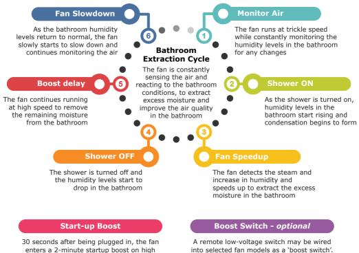
speed to ensure bad or stale air is removed from the bathroom, before the fan slowly slows down and begins its Bathroom Extraction Cvcle
